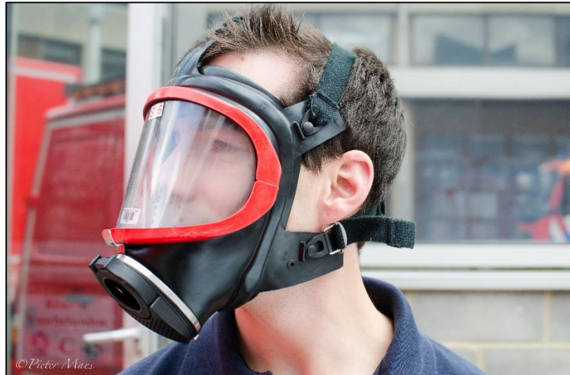
figure 4 A rescue mask which can be put on the victim's head. A regulator or lung demand valve has to be attached, preferably with an extra-long hose so that both victim and firefighter can move easily alongside each other. (Photo: Pieter Maes)
