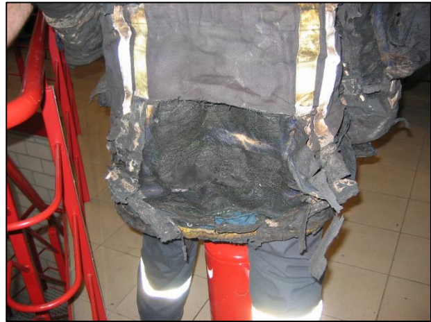
figure 3 This is the turnout jacket of one of the firefighters. It has been heavily damaged. (Photo: Fire service Westhoek – station Diksmuide)
