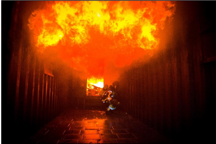
figure 6 A firefighter involved in a training run for studying fire gas ignitions. When he opens the door at the back end, the smoke layer at the ceiling ignites due to the exiting flames. The firefighter is subject to a very high radiant heat during this training. (Photo: Stijn Hermans)
