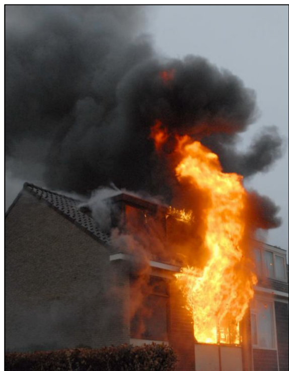
Figure 5 Fully developed fire venting from the back of a building. (Photo: nufoto.nl)
