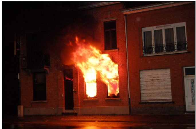
Figure 3 Fully developed fire on the ground floor. This fire can be tackled using an indirect attack. Suppose the fire is located on the first floor or higher, a short exterior attack with a full jet against the ceiling may then offer the solution. (Photo: Nico Speleers)
