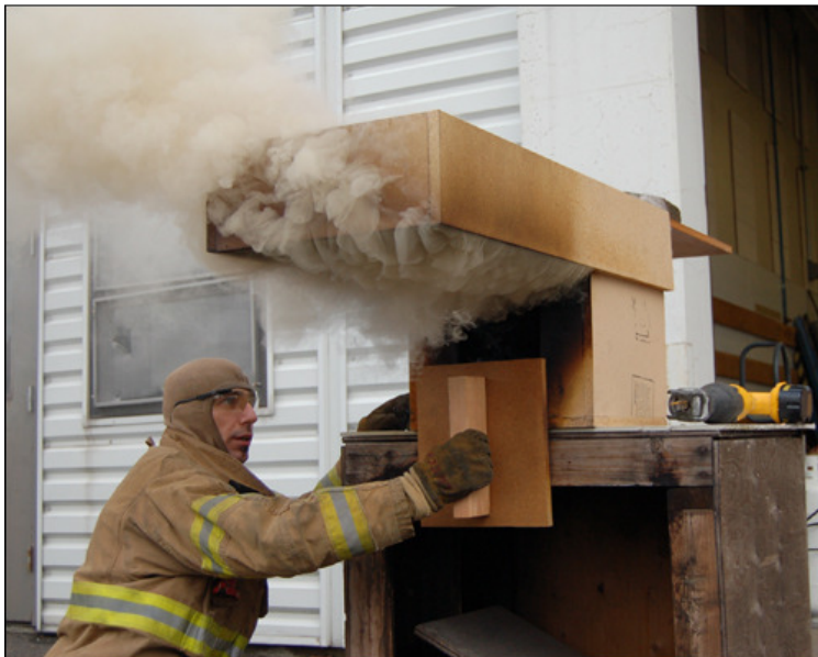
Fig 1.1 The compartment at the back is burning. Smoke gas has leaked from the closed off door and has formed an explosive mixture up against the ceiling (Photo: Ed Hartin)
