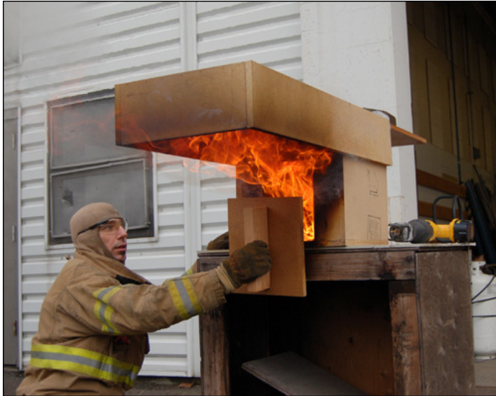
Fig 1.3 Fully developed fire after a flash fire. (Photo: Ed Hartin)
