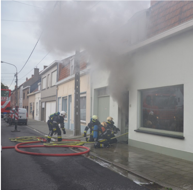
Figure 4 Double flow for a compartment fire. Smoke is flowing out from the top of the door opening. Air is flowing in from the bottom. (Photo: Nico Speleers)
