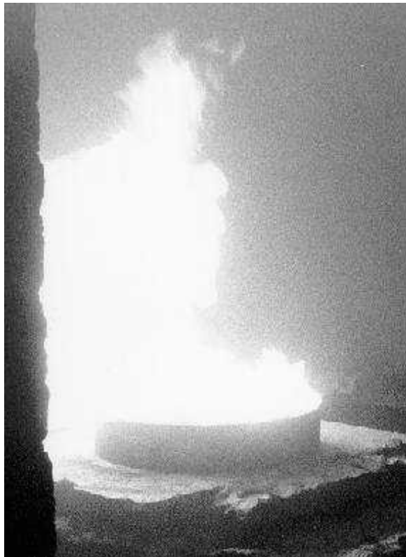
Figure 16. Photo from test 10 showing inclination and turbulence of the flame due to positive pressure ventilation. Photo taken, by author, from door D2 looking into Room 2, without using breathing apparatus.
