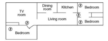
Figure No. 6 In family living units with more than one sleeping area, a smoke detector should be provided to protect each sleeping area in addition to detectors required in bedrooms. (Figure A-8-1.2.1(b) from NFPA 72)
