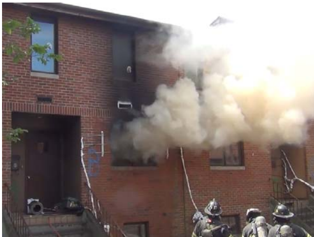
Figure 4.39: Flow path out re-established after Stream was Shut Down
