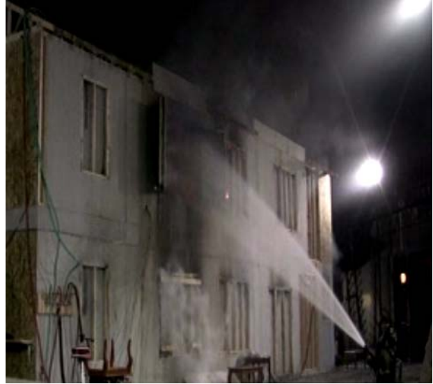
Figure 4.36: Fog Stream Sealing Flow Path
