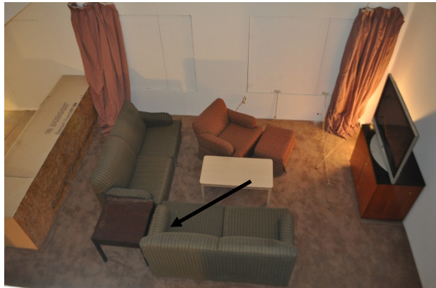
Figure 3.15: Two-Story Family Room Ignition Location
