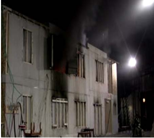
Figure 4.35: Flow path before Water Application
