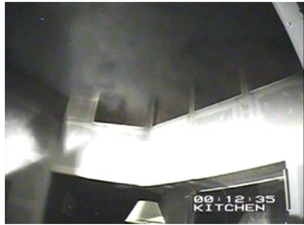
Figure 4.31: Five seconds into water application, visible flame out
