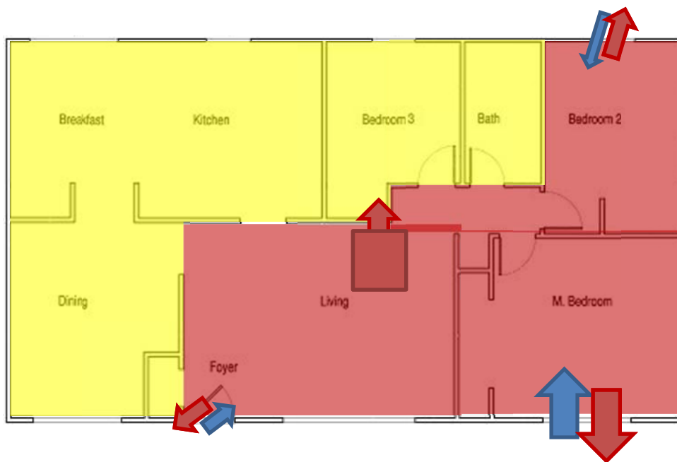
Figure 4.20: Flow paths as fire becomes fully developed
