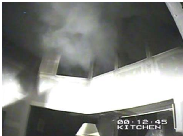
Figure 4.32: At end of water application, steam moving to roof vent
