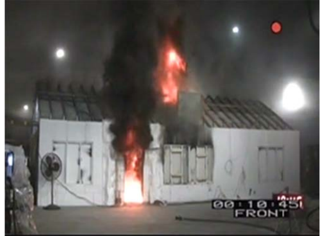
Figure 4.6: 60 seconds after roof vent
