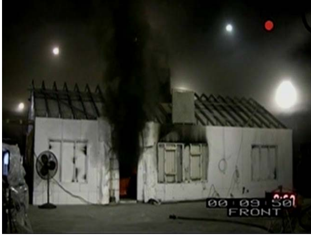
Figure 4.5: 5 seconds after roof vent
