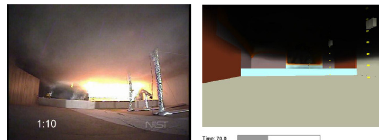
Figure 5-9. Smoke layer has dropped to 1.5 m above floor, t = 70 seconds after ignition.
